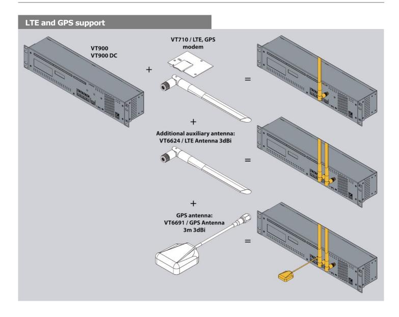
"VT710 / LTE, GPS modem" provides ethernet over LTE. Can work as a router. Adds time over GPS. Allows to receive and send messages. Ordered separately. Possible to order additional auxiliary for more stable signaland GPS antennas.
