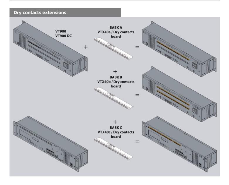
The unit has a built-in "VTX16 / Dry contacts board" which includes x16 dry contact inputs (two wire interface). Used for contacts of windows, doors, fire / burglar alarms, power systems, exit / push buttons. VTX16 is supplied by default.
